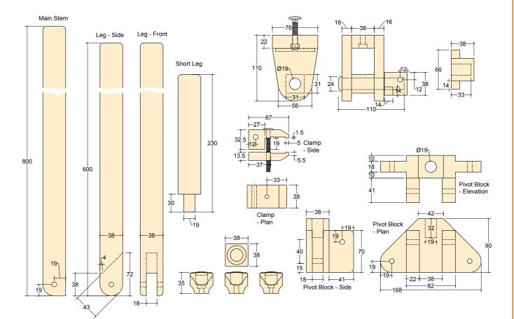
Next, cut the end off the board, leaving 620mm for the remaining sticks and allowing for a final trim. Cut the two legs and a stick for the other bits from the 620mm section. To make it easier to round over the ends of the legs, make small 45° cuts to remove most of the waste.
